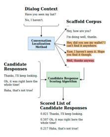
Fig. 2. Workflow diagram: The dialog context is converted to an array of sentence embeddings using Google's Universal Sentence Encoder, then passed to an embedded concatenation localization function to determine the best contextual match(es). The matched utterances (orange) along with their direct successors (red) are then passed to the Response Scoring Algorithm, which assigns a numerical value to each candidate response. Image originally published in [27]. (Color figure online)
